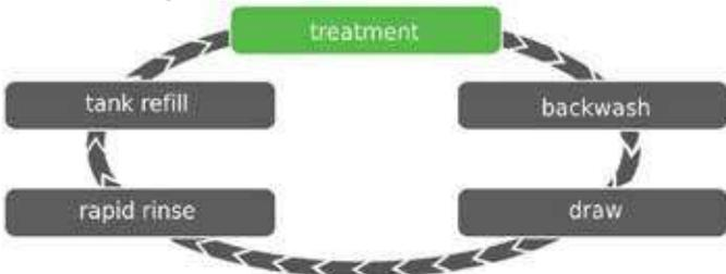
**NOTE: On metered units, the "Treatment" step on the Regeneration Cycle Wheel will flash when water is flowing through the unit.**
